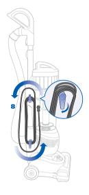
**6** Attach each end of the Super Stretch Hose to the vacuum and press into Upper Hose Holder for easy storage.
