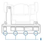
Turn the three locking screws clockwise (i) to tighten.
