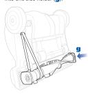
Partially insert the left end into the other side holder (h).
