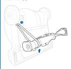
Partially insert the right end of the roller into one side holder (a).
