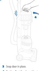
4 Position Dust Cup Assembly at a forward angle over unit and then snap into place.
