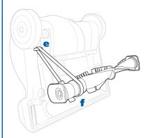
Partially insert the right end of the roller into one side holder (g).
