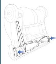
Center Belt on motor-driven shaft; test Brush Roll for easy turning.
