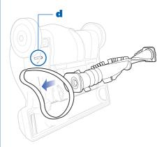
With the Brush Roll free, inspect for any hair build-up or string; if present, carefully cut out with scissors; take care not to damage the bristles.
