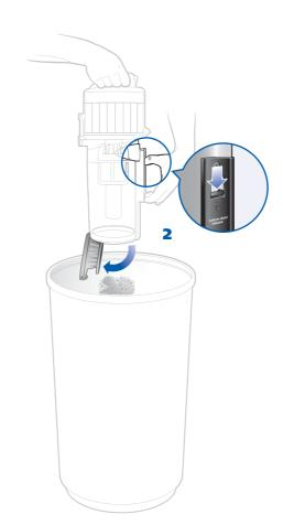
2 Insert Dust Cup Assembly deep inside trash receptacle to contain dust and debris.
