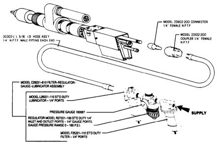
Your ARO Self-Feed tool is designed to deliver specific horsepower and thrust to achieve high rates of work. To assure the unit will develop this power, care must be taken that the power air inlet system is correctly sized to permit the proper rate of air flow. Shown is a system for a single tool that will supply correct delivery. IMPORTANT — the tool is power rated when 90 P.S.I. is present AT THE TOOL DURING OPERATION.
