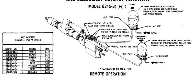
Remote operation of the unit may be achieved by connecting a 3-way valve to the remote start and/or remote retract ports, as shown above.
