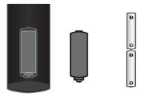
2 Insert two AAA batteries (included) into the battery compartment. Make sure that the + and – symbols on the batteries match the + and – symbols in the battery compartment.
