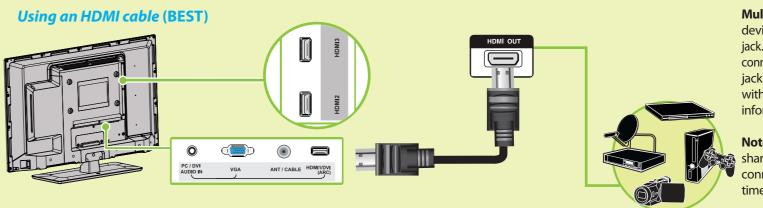
**Multipurpose jacks:** You can plug any device that uses HDMI into any HDMI jack. However, certain devices must be connected to the **HDMI1/DVI (ARC)** jack. See the instructions that came with your ARC or DVI device for more information.
