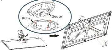
3 Align the stand cover with the stand column, then secure the stand cover to the stand column with one M5 x 12 mm screw (provided). Make sure that the bottom of the stand cover is flush against the top of the stand column.
