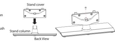
**4** Secure the stand cover to the TV screen using four M5 x 12 mm screws (provided).
