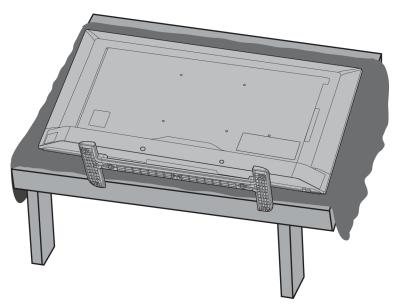
2 If the TV stand is attached, remove the four screws that secure the stand to the TV, then remove the stand.
