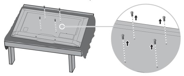
**4** Attach the wall-mount bracket using the screws you removed or the screws that came with the wall-mount bracket. See the instructions that came with the wall-mount bracket for information about which screws to use and how to correctly hang your TV.
