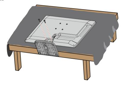
**3** Attach the wall-mount bracket to your TV using the mounting holes on the back of your TV. See the instructions that came with the wall-mount bracket for information about how to correctly hang your TV.
