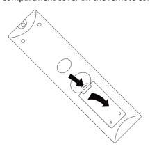
2 Insert two AAA batteries into the battery compartment. Make sure that you match the + and – symbols on the batteries with the + and – symbols in the battery compartment.
