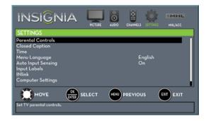
3 Press ▲ or ▼ to highlight **Parental Controls**, then press **ENTER**. The *Enter password* screen opens.
