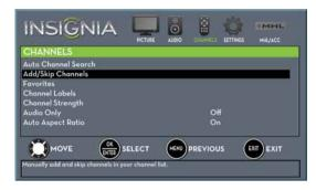
3 Press ▲ or ▼ to highlight Add/Skip Channels, then press ENTER. The CHANNELS · ADD/SKIP CHANNELS screen opens.
