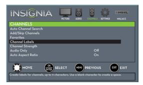
3 Press ▲ or ▼ to highlight **Channel Labels**, then press **ENTER**. The *CHANNELS* · *CHANNEL LABELS* screen opens.
