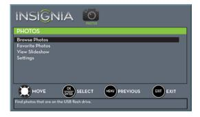
2 Press ▲ or ▼ to highlight **Browse Photos**, then press **ENTER**. The screen displays folder names and photo files stored on the USB flash drive in a thumbnail index with the first folder or file highlighted. A control bar appears at the bottom of the screen.
