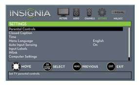
3 Press ▲ or ▼ to highlight **Parental Controls**, then press **Enter**. The *Enter password* screen opens.
