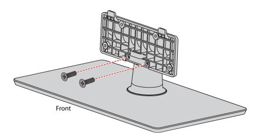
**6** Secure the stand cover to your TV using four provided M5  $\times$  12 mm screws.
