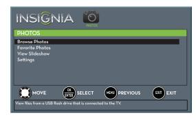
2 Press ▲ or ▼ to highlight Browse Photos, then press ENTER. The screen displays folder names and photo files stored on the USB flash drive in a thumbnail index with the first folder or file highlighted. A control bar appears at the bottom of the screen.
