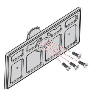
4 Slide the stand cover onto the stand column, then secure the back of the cover to the column using two provided M5  $\times$  12 mm screws.
