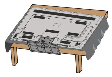
2 If the TV stand is attached, remove the four screws that secure the stand cover to the TV, then remove the stand.
