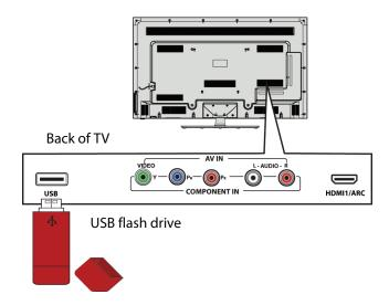
1 Plug a USB flash drive into the **USB** port on the back of your TV.
