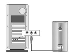
3 Plug the black plug from the AC adapter into the back of the right speaker and the other end into a wall outlet or power strip.
