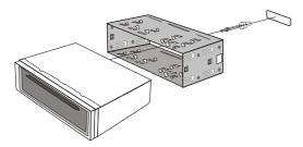
**6** Secure the rear mounting bolt to the firewall or other sturdy support using the back strap (if necessary).
