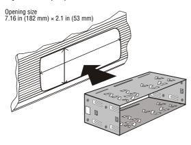
2 When the mounting sleeve is in the correct position, bend several mounting *claws* outward to achieve a tight fit and lock the mounting sleeve into place.
