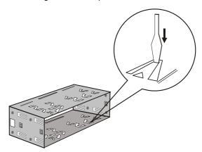
3 Install the outer trim frame on the CD deck.
