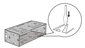
3 Install the outer trim frame on the CD deck.
