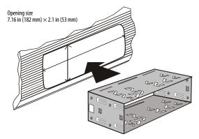
2 When the mounting sleeve is in the correct position, bend several mounting *claws* outward to achieve a tight fit and lock the mounting sleeve into place.
