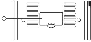
2 Insert two (2) AAA batteries into the battery compartment. Make sure that you match the + and – symbols on the batteries with the + and – symbols in the battery compartment.
