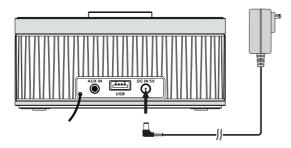
**2** Plug the other end of the AC power adapter into a power outlet.
