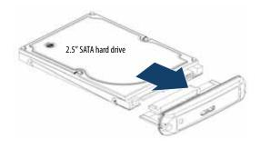
4 Gently slide the drive tray, with drive attached, into the enclosure.
