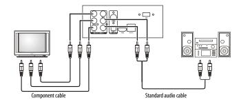
2 Connect a standard audio cable (not provided) to the L and R AUDIO OUT jacks on the back of your TV, then connect the other end of the cable to the corresponding AUDIO IN jacks on the sound system.
