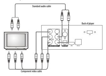
2 Connect a standard audio cable (not provided) to the L and R AUDIO OUT jacks on the back of your player, then connect the other end of the cable to the corresponding AUDIO IN jacks on the component TV.
