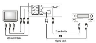
2 Connect a coaxial digital audio cable (not provided) to the COAXIAL DIGITAL AUDIO OUT jack on the back of your player, then connect the other end of the cable to the COAXIAL IN jack on the sound system.
