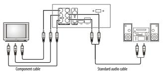
2 Connect a standard audio cable (not provided) to the L and R AUDIO OUT jacks on the back of your TV, then connect the other end of the cable to the corresponding AUDIO IN jacks on the sound system.
