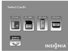
2 Insert a new memory card or press ◀ or ► to select the built-in memory or existing memory card.
