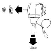
**2** Slide the stand into the hole at the center of the base, then tighten the pole locking cap underneath the base.
