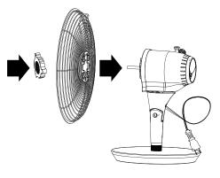
**4** Put the fan blade on the motor shaft, then screw the blade cap on to hold it in place. Make sure that the stem of the fan blade is closest to the motor housing.
