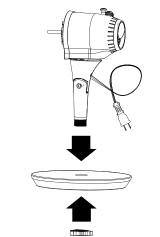
**3** Slide the back guard onto the motor shaft, then screw the guard knob on to hold it in place. Make sure that the handle is at the top.
