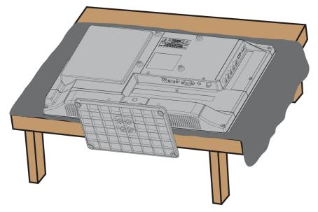
2 If the stand is attached, remove the three screws that secure the stand column to the TV, then remove the stand column.
