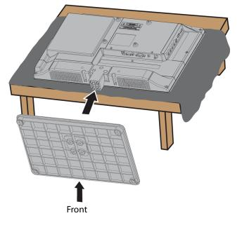
**3** Secure the TV stand to the TV with the four provided screws.
