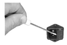
The fuse holder contains a spare fuse as shown. To reinstall just snap the new fuse in place and snap the fuse holder back into the IEC connector.
