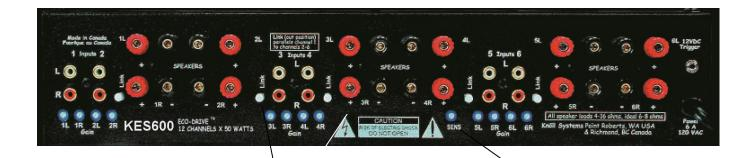
The Link button is normally set to the in position to give all six stereo inputs individual sources. When a channel Link button is set to the out position, that channel is (Left/Right) linked or cascaded to input #1 (without the use of Y cords). Any or all combinations of linked inputs 2 to inputs 6 are possible. When all inputs are linked to input one, the input impedance is about 8500 ohms.
