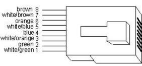
are connected using a single cat 5 wire using all 8 conductors. Connection is made with the RJ45 connector (RJ45 plug not supplied). Always use standard cat 5 wiring practices. Using the correct wire pairs and polarity is **VERY** important.
