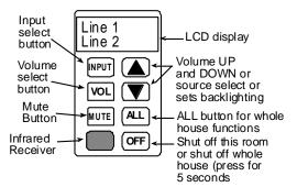
Adjusting Backlighting. MR164's are backlit for easy nighttime operation. To adjust the backlighting make sure the power for the keypad is
