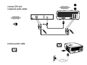
Connect the power cord to the **Power** connector on the side of the projector and to your electrical outlet.
