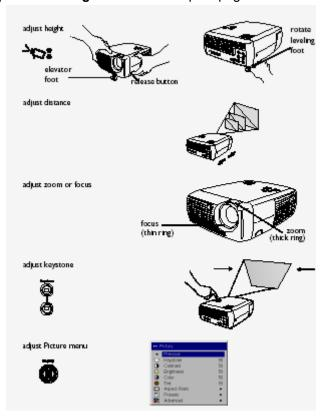
Press the top **Keystone** button to reduce the upper part of the image, and press the bottom **Keystone** button to reduce the lower part.
