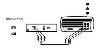
Plug a white connector into the left audio out connector on the video device and plug a red connector into the right audio out connector on the video device. Plug the remaining white connector into the white **audio in c**onnector on the projector, and plug the remaining red connector into the red **audio in** connector on the projector.
