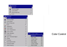
Video Standard: when it is set to Auto, the projector attempts to automatically pick the video standard based on the input signal it receives. (The video standard options may vary depending on your region of the world.) If the projector is unable to detect the correct standard, the colors may not look right or the image may appear "torn." If this happens, manually select a video standard by selecting NTSC, PAL, or SECAM from the Video Standard menu.
