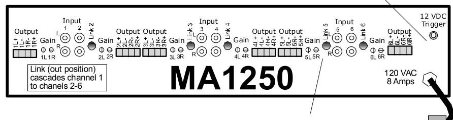
Caution: NEVER connect the MA1250 to impedances less than 4 ohms or amplifier damage not covered by the warranty may occur.
