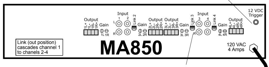
Caution: NEVER connect the MA850 to impedances less than 4 ohms or amplifier damage not covered by the warranty may occur.
