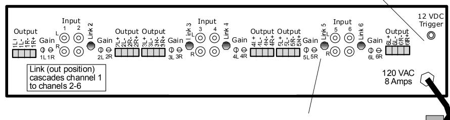
Caution: NEVER connect the MR1250f to impedances less than 4 ohms or amplifier damage not covered by the warranty may occur.
