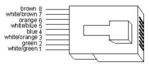
a single cat 5 wire using all 8 conductors. Connection is made with the RJ45 connector (RJ45 plug not supplied). Always use standard cat 5 wiring practices. Using the correct wire pairs and polarity is **VERY** important.
