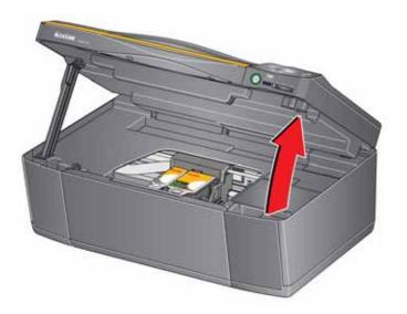
The ink cartridges are located in the printhead.
