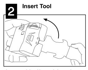
Insert special tool into end slot as shown.
