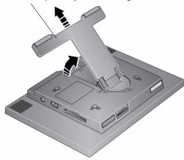
When displayed with the stand extended, the frame rests at a 68-90 ° angle.
