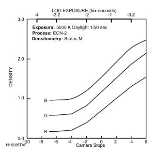
The curves describe this film's response to red, green, and blue light. Sensitometric curves determine the change in density on the film for a given change in log exposure.<sup>3</sup>
