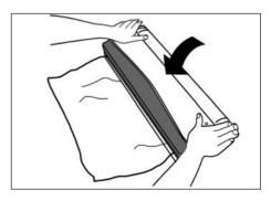
Press and hold the Seal/Cut button () with both hands until the control lamp () lights up.
