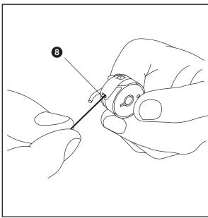
3 until the thread passes out of the slit in the bobbin case.
