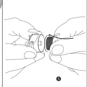
5 Wind about 10 cm of thread away from the bobbin and feed this into the bobbin case.
