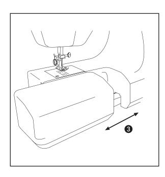
3 The box compartment can now be simply pushed back in, for example if you need it as an 'extension flap' for sewing larger areas of material. However, you can also leave the box detached, for example forfree-arm sewing on sleeves, trouser legs, etc.
