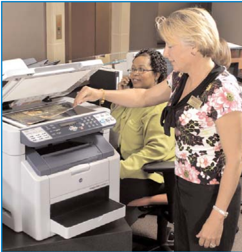
Both the flatbed and the automatic document feeder accept documents up to 8.5" x 14".
