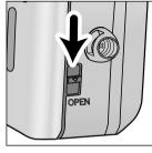
1. Slide the back-cover release down to open the back cover.
