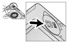
1. Open the battery-chamber door by sliding the battery-chamber release in the direction indicated.
