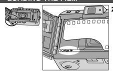
2. Place the film cartridge into the film chamber. Extend the film leader to the "FILM TIP" mark, making sure it lays flat.
