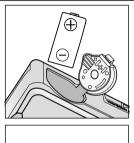
2. Insert the battery matching the positive terminal mark inside the battery chamberdoor, then click the door closed.
