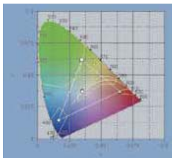
Pass/fail judgment using polygon tolerance (limit values) setting on a chromaticity diagram
