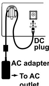
Pass the AC adapter cord through the cord hook so that the plug won't be removed from the jack accidentally. When you unhook the cord, don't pull the cord with force.
