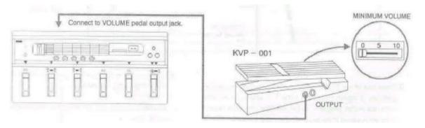
Use the KORG KVP 001 volume pedal. Connect the output jack (OUTPUT) of the KVP 001 into the VOLUME pedal jack (PEDAL) of the A5 GUITAR (Also make sure that the KVP 001 slider has been set to the minimum volume of "0").
