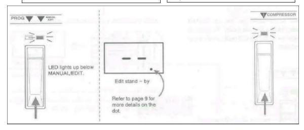
In the Manual/Edit mode, the EFCT/PROG switches (along with the EFCT/PROG LEDs) control ON/OFF of each of the five effects. When entering the Manual/Edit mode the EFCT/PROG LEDs light up to display the effects which are currently turned on. For example the figure below shows that the Manual/Edit mode is selected after selecting METAL 1" in the Program mode.
