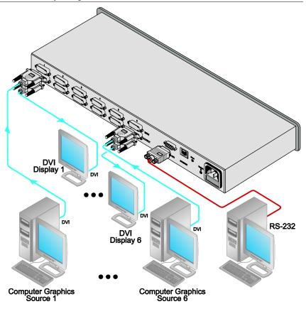
Figure 2: Connecting the VS-66HDCP 6 x 6 DVI Matrix Switcher
