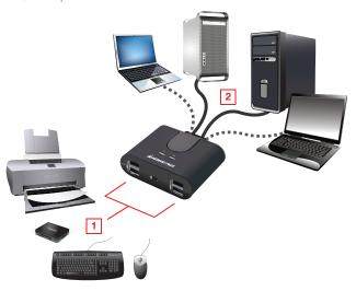
Note: The GUS402/GUS404 are hot-swappable and do not require the computers to be turned off during connection, or when attaching devices to the USB ports.
