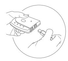
• Cable from the USB peripheral can be plugged into any available port.
