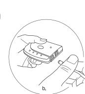
1. Plug the power adapter into the AC source, then plug the power adapter cable  $\,$ into the unit's power jack.
