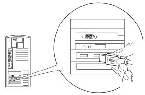
3. Plug the Hi-Speed USB 2.0 Cable (type A end) into your computers Hi-Speed USB 2.0 Port.
