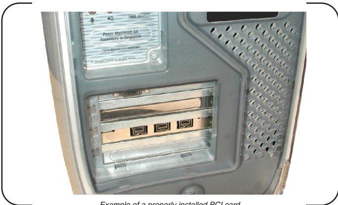
Example of a properly installed PCI card.
