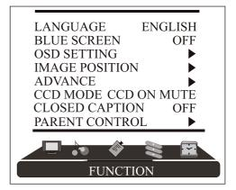
2 Press CH- or CH+ to select PARENT CONTROL, then press VOL- or VOL+. The Password box opens.
