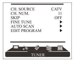
2 Press CH- or CH+ to select CH.SOURCE, then press VOL- or VOL+ to choose CATV or AIR.
