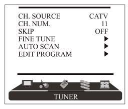
2 Press CH- or CH+ to select EDIT PROGRAM, then press VOL- or VOL+ to enter the sub-menu. The *Edit Program* sub-menu opens.
