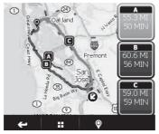
The color of the route option box corresponds to the color of the route on the map. Touch the destination pointer at the bottom right of the screen to zoom in to the destination.
