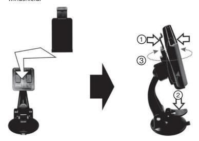
**4** Rotate the mounted GPS (3) to a comfortable viewing position.
